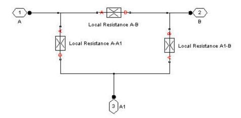
To specify pressure loss for all possible flow directions, you have to provide six pressure loss coefficients. The flow regime is checked in the underlying Local Resistance blocks by comparing the Reynolds number to the specified critical Reynolds number value, and depending on the result, the appropriate formula for pressure loss computation is used. For more information, see the reference documentation for the Local Resistance block.
