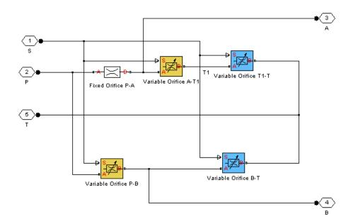
All Variable Orifice blocks are controlled by the same position signal, provided through the physical signal port S, but the **Orifice orientation** parameter in the block instances is set in such a way that positive signal at port S opens the orifices colored blue in the block diagram (orifices A-T1 and P-B) and closes the orifices colored yellow (orifices T1-T and B-T). As a result, the openings of the orifices are computed as follows:
