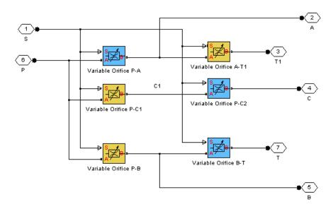
All blocks are controlled by the same position signal, provided through the physical signal port S, but the **Orifice orientation** parameter in the block instances is set in such a way that positive signal at port S opens the orifices colored blue in the block diagram (orifices P-A, B-T, and P-C2) and closes the orifices colored yellow (orifices A-T1, P-B, and P-C1). As a result, the openings of the orifices are computed as follows:
