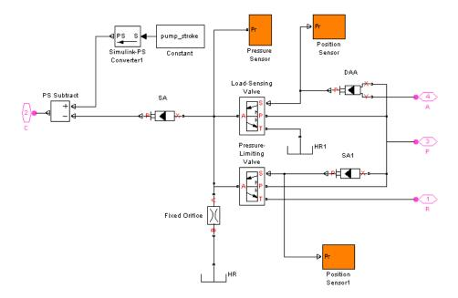
There are three hydraulic valve actuators in the model:
