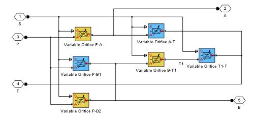
All Variable Orifice blocks are controlled by the same position signal, provided through the physical signal port S, but the **Orifice orientation** parameter in the block instances is set in such a way that
