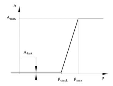
The valve remains closed while pressure differential across the valve is lower than the valve cracking pressure. When cracking pressure is reached, the value control member (spool, ball, poppet, etc.) is forced off its seat, thus creating a passage between the inlet and outlet. If the flow rate is high enough and pressure continues to rise, the area is further increased until the control member reaches its maximum. At this moment, the valve passage area is at its maximum. The valve
