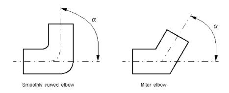
Therefore, the pressure loss coefficient for smoothly curved, standard elbows is determined with the formula
