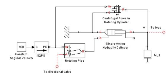
The centrifugal force generated by the Centrifugal Force in Rotating Cylinder block sums up with that of the cylinder at node A. The Rotating Pipe block simulates the pipeline between the cylinder chamber and the channel in the center of a rotating shaft where the cylinder is installed.
