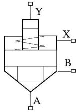
The actuator drives a valve (spool, poppet, and so on) whose position depends on pressures at ports A, B, X, and Y and the spring force. Pressures at ports A and B tend to open the valve, while pressures at control ports X and Y, together with the spring force, act to close it. The model does not account for flow consumption and loading forces, except spring and pressure forces.
