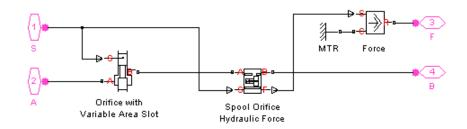
It consists of an Orifice with Variable Area Slot block, which simulates hydraulic properties of the orifice, connected in series with a Spool Orifice Hydraulic Force block. The force value computed in the block is exported through its port F and passed to the Force block.
