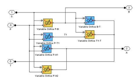
All Variable Orifice blocks are controlled by the same position signal, provided through the physical signal port S, but the **Orifice orientation** parameter in the block instances is set in such a way that positive signal at port S opens the orifices colored blue in the block diagram (orifices P-A1, P-T1, and B-T) and closes the orifices colored yellow (orifices P-A2, P-B, and T1-T). As a result, the openings of the orifices are computed as follows:
