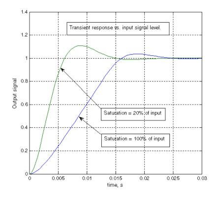
You can adjust the block parameters, such as saturation, gain, and time constant, to make the transient responses close enough to those provided in the data sheet. The most effective way to adjust the parameters is to use the Optimization Toolbox<sup>TM</sup> software.
