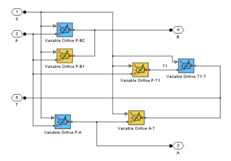
All Variable Orifice blocks are controlled by the same position signal, provided through the physical signal port S, but the **Orifice orientation** parameter in the block instances is set in such a way that positive signal at port S opens the orifices colored blue in the block diagram (orifices P-B2, P-A, and T1-T) and closes the orifices colored yellow (orifices P-B1, P-T1, and A-T). As a result, the openings of the orifices are computed as follows:
