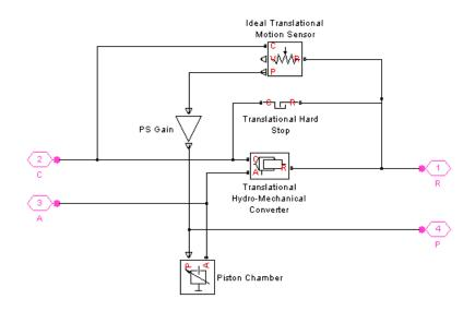
Connections R and C are mechanical translational conserving ports corresponding to the cylinder rod and cylinder clamping structure,
