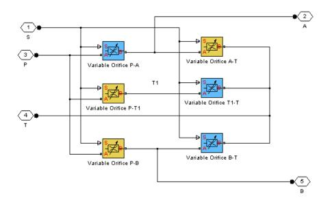
All blocks are controlled by the same position signal, provided through the physical signal port S, but the **Orifice orientation** parameter in
