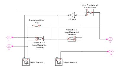
Connections R and C are mechanical translational conserving ports corresponding to the cylinder rod and cylinder clamping structure, respectively. Connections A and B are hydraulic conserving ports. Port A is connected to chamber A and port B is connected to chamber B.
