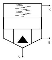
The Cartridge Valve Insert block is a structural model consisting of a Hydraulic Cartridge Valve Actuator block and a Variable Orifice block, as shown in the next illustration.
