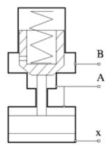
Unlike a conventional check valve, the pilot-operated check valve can be opened by inlet pressure  $p_A$ , pilot pressure  $p_X$ , or both. The force acting on the poppet is determined as
