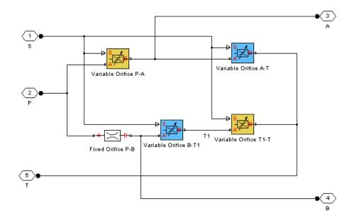
All Variable Orifice blocks are controlled by the same position signal, provided through the physical signal port S, but the **Orifice orientation** parameter in the block instances is set in such a way that positive signal at port S opens the orifices colored blue in the block diagram (orifices B-T1 and A-T) and closes the orifices colored yellow (orifices P-A and T1-T). As a result, the openings of the orifices are computed as follows:
