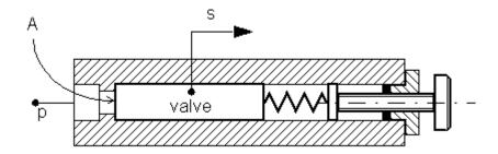
The actuator consists of a piston and a spring. The spring, which can be preloaded, tends to keep the piston at the initial position. As pressure applied to the piston develops enough force to overcome the spring preload, the piston moves to the opposite position until it reaches its maximum stroke.
