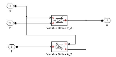
One Variable Orifice block, called orifice\_PA, is installed in the P-A path. The second Variable Orifice block, called orifice\_AT, is installed in the A-T path. Both blocks are controlled by the same position signal, provided through the physical signal port S, but the **Orifice** orientation parameter in the block instances is set in such a way that positive signal at port S opens orifice\_PA and closes orifice\_AT. As a result, the openings of the orifices are computed as follows:
