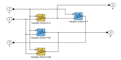
All Variable Orifice blocks are controlled by the same position signal, provided through the physical signal port S, but the **Orifice orientation** parameter in the block instances is set in such a way that
