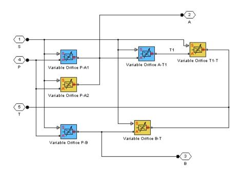
All Variable Orifice blocks are controlled by the same position signal, provided through the physical signal port S, but the **Orifice orientation** parameter in the block instances is set in such a way that positive signal at port S opens the orifices colored blue in the block diagram (orifices P-A1, A-T1, and P-B) and closes the orifices colored yellow (orifices P-A2, B-T, and T1-T). As a result, the openings of the orifices are computed as follows:
