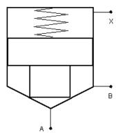
The Cartridge Valve Insert block is a structural model consisting of a Hydraulic Cartridge Valve Actuator block and a Poppet Valve block, as shown in the next illustration.
