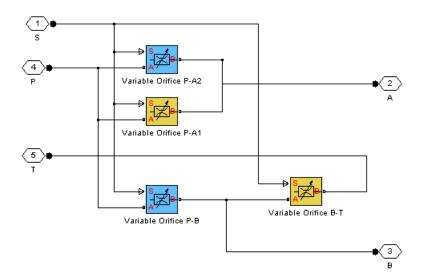
All Variable Orifice blocks are controlled by the same position signal, provided through the physical signal port S, but the **Orifice orientation** parameter in the block instances is set in such a way that positive signal at port S opens the orifices colored blue in the block diagram (orifices P-A2 and P-B) and closes the orifices colored yellow (orifices P-A1 and B-T). As a result, the openings of the orifices are computed as follows:
