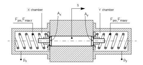
As pressure applied to the piston develops enough force to overcome the spring preload, the piston moves to the opposite position until it reaches its maximum stroke. Pressure applied at port X shifts the valve in the x-direction, overcoming the spring located in the Y chamber. Pressure
